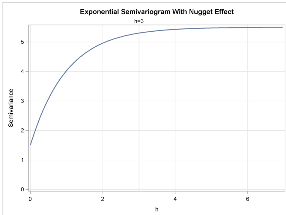
Figure 68.11 Exponential Semivariogram Model with a Nugget Effect c_n = 1.5
